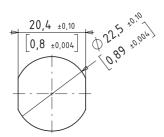
The SENSORswitch is secured against rotation by the illustrated hole. Metric and imperial measurements are used in drawings. Imperial measurements are marked with [ ].
