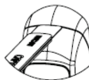
Removal of the HWT2 cup Special tool „HWT2-DW“
